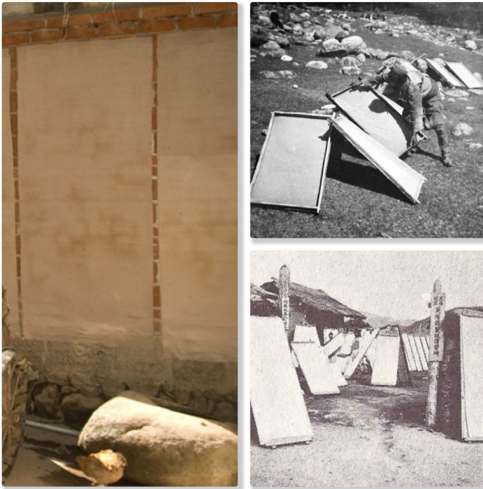
Figs 4 A-C. A. Drying support: Left on a wall. Photograph courtesy of Claude Laroque; B. Top: on a mould. Photograph by Jesper Trier; C. Bottom: On a wooden plank. Photograph after Dard Hunter
