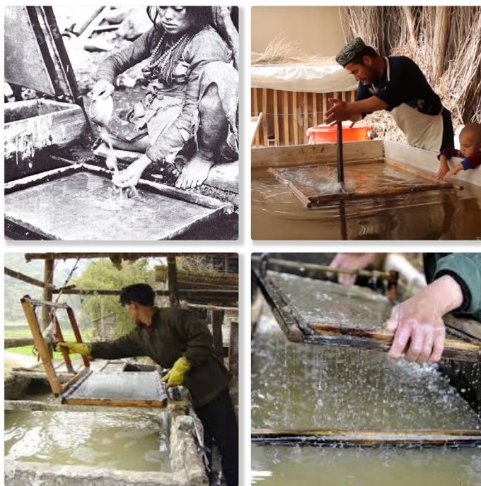
Figs 3 A-D. The two main sheet shaping processes. Top A and B: Floating mould, pulp is spread manually (left) or by means of a tool (right). Bottom C and D: Dipping mould from Japan (left) and China (right). Photographs A by Trier, B by Josh Summers, bottom C and D www.cnnews.com
