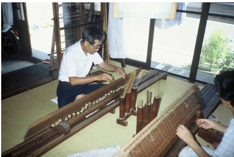
Fig. 16. Production of screens of bamboo splints and twisted silk threads
