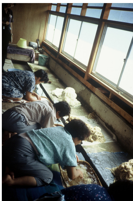
Fig. 15. Careful sorting in water of the kōzo fibres before the mechanical maceration
