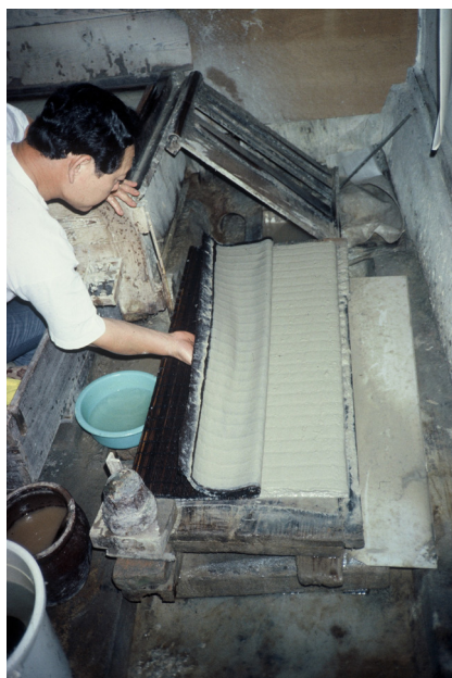
Fig. 10. Final couching of gampi sheet of paper on the horizontal stack
