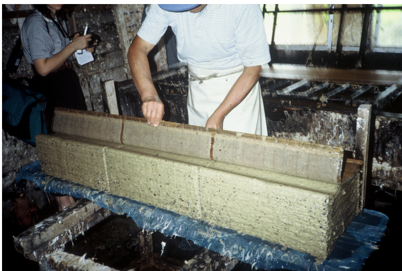
Fig. 6. Couching the sheet of paper with the help of the removable, flexible screen on the paper stack.
