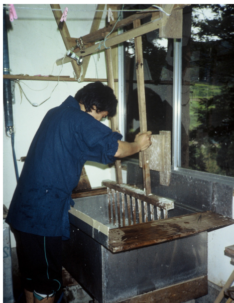
Fig. 12. Mixing pulp and mucilage with the reed before the formation of the sheet takes place
