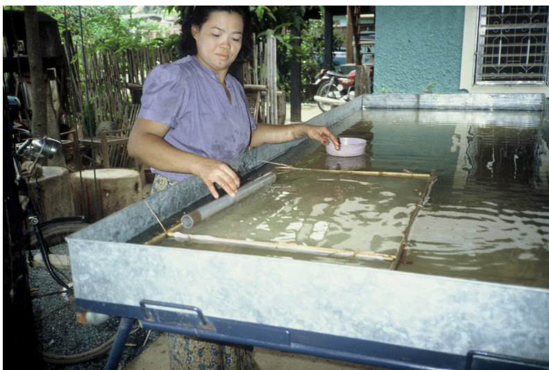
Fig. 5. Khoi floating mould technology is used, but paper mulberry fibres are chosen instead of Khoi fibres
