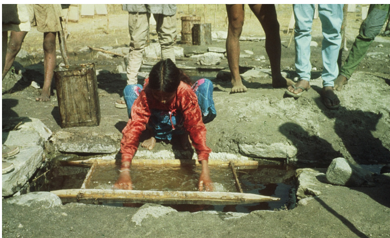
Fig. 13. Manual distribution of the pulp of lokta fibres within the floating mould (Photo: Paper maker Prem Bahadur Lama, 1984)
