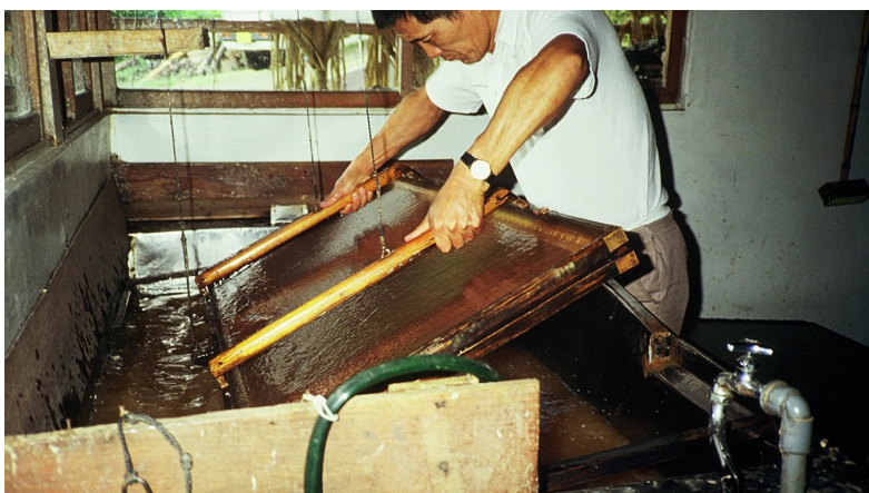
Fig. 11. Scooping mitsumata pulp with the hinged dipping mould
