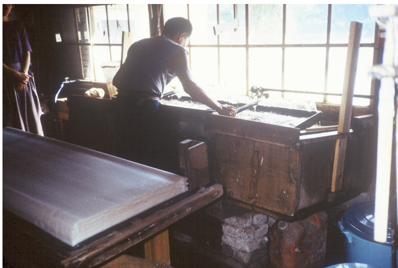
Fig. 17. Sheet formation of tengujoshi paper
